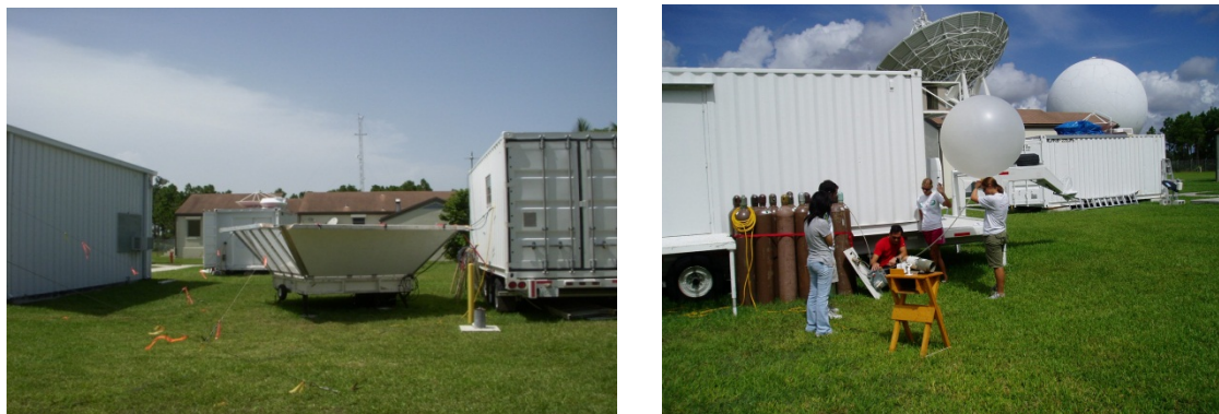
Figure 2.2: Photos of instrumentation from the field site at CSTARS. The picture on the left shows the wind profiler (MAPR) in the center of the image, the NCAR container to the right, and the UM container with the X-band and W-band antennas in the background. The right image shows scientists preparing to launch a rawinsonde in front of the NCAR container.
